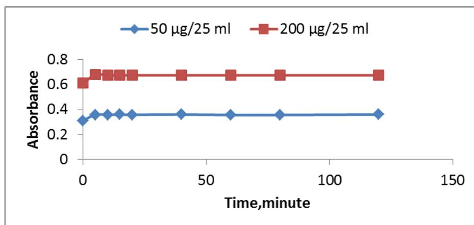
Fig. 5: Effect of time and amount of SMX on absorbance.
