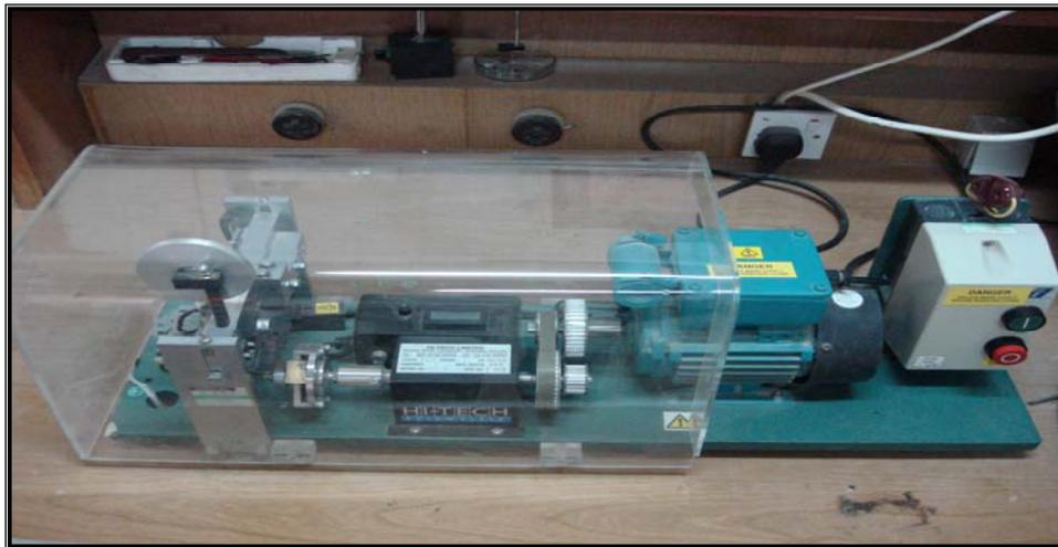
**Fig. 1: Bending fatigue machine**
