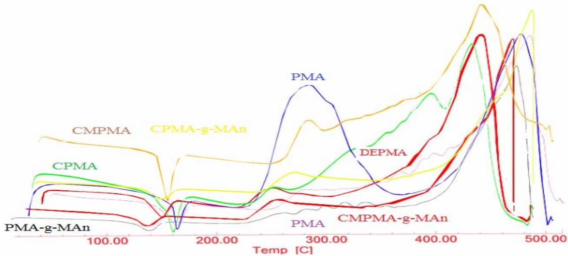
**Fig. 1: DSC –Thermogram of the grafted polymer**
