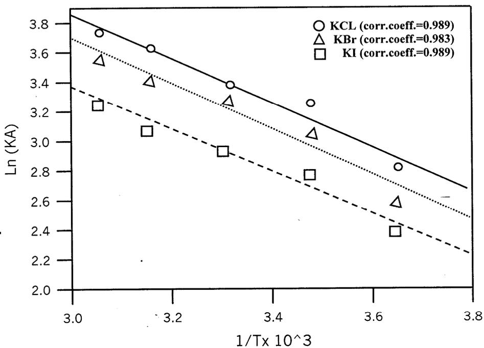
Fig:4: ire 4 The plot of  $\ln(K_A)$  against the KCL, KBr and KI electrolytes in methanol.
