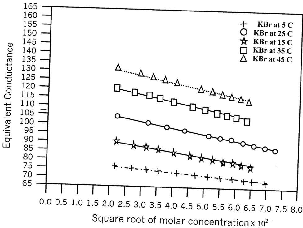
Fig:2: 2 the plot of equivalent conductance against the molar concentration for KBr in methanol at different temperatures
