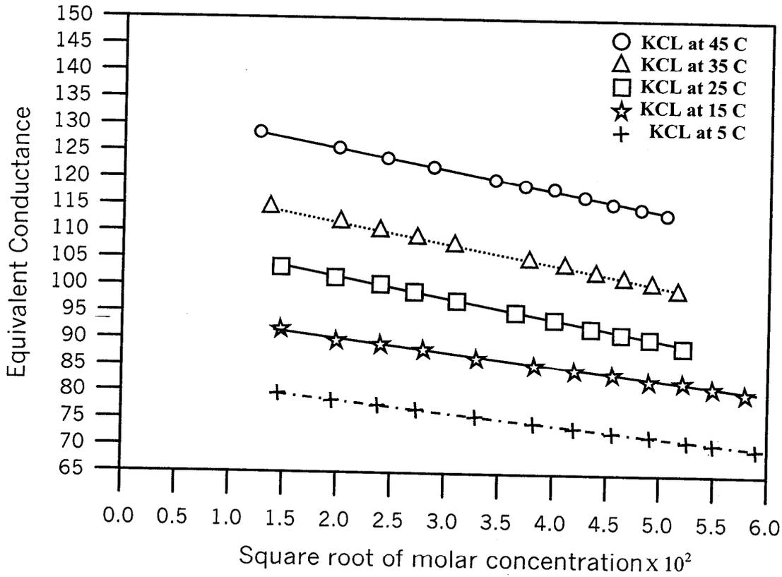
Fig:1: e 1 the plot of equivalent conductance against the square root of molar concentration for KCL at different temperatures
