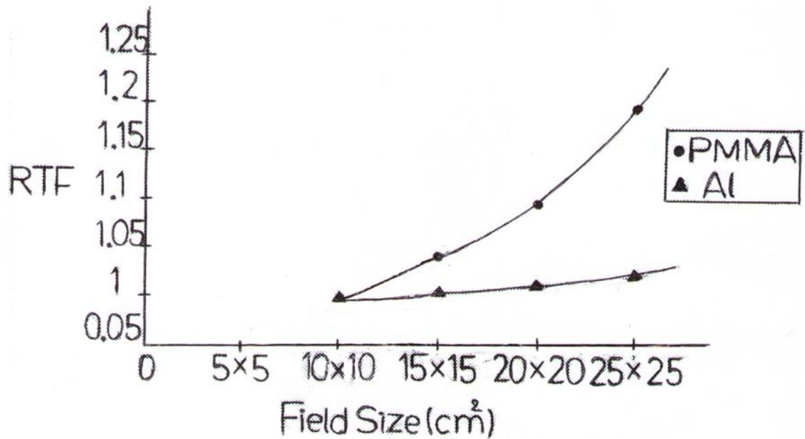
Fig. 3: RTF as a function of field sizes and SSDs for PMMA and Al tray, SSD= 70 cm.
