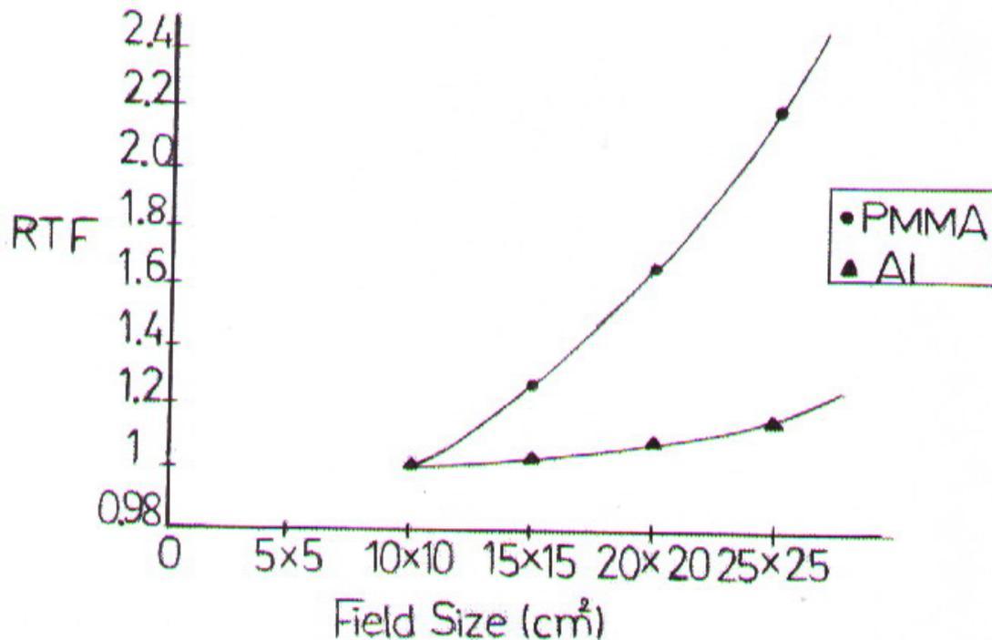
Fig. 2: RTF as a function of field sizes and SSDs for PMMA and Al tray, SSD= 60 cm.
