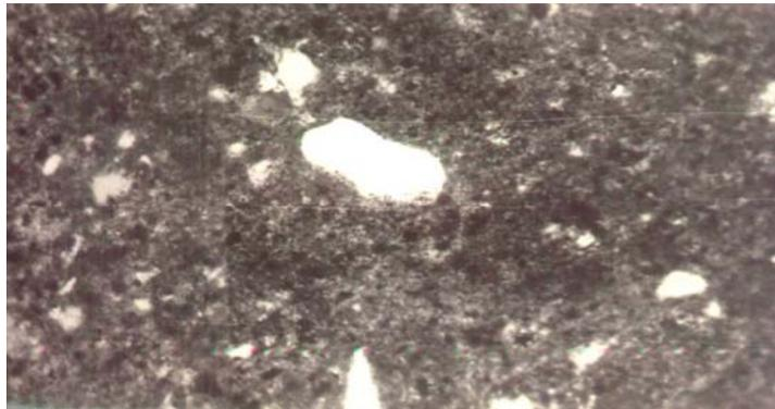
Plate 2 : Quartz Grains Showing Reaction Rims (centre)
