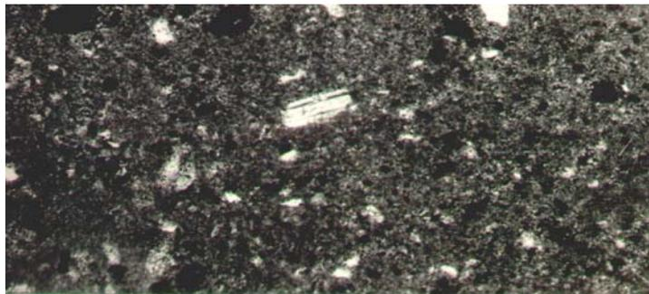
Plate 3 : Plagioclase Feldspars (centre) with Lamellar twinning and Reaction Rim.
