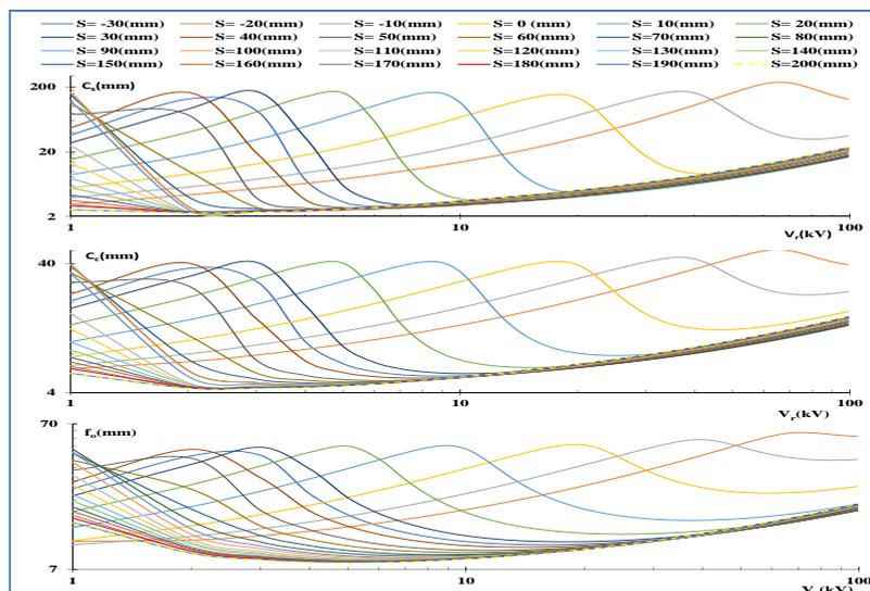
**Fig. 4: Comparison of the values of  $C_s$ ,  $C_c$  an  $f_o$  as a function of the accelerating voltage calculated at different values of S.**
