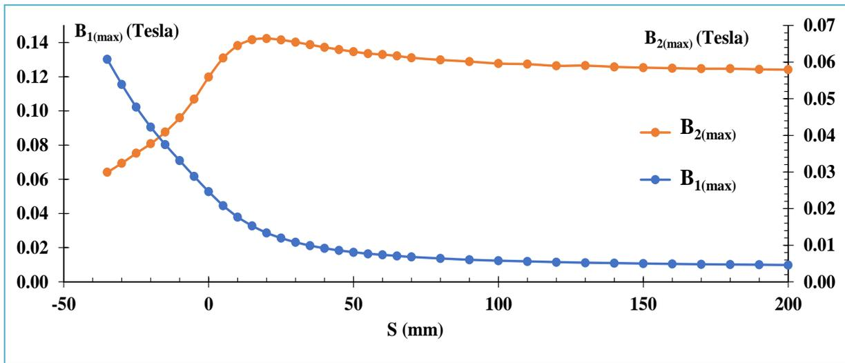
**Fig. 3: Comparison between the values of  $B_{1(Bmax)}$  for low peak and  $B_{2(Bmax)}$  for high peak of the lens at different values of (S), calculated at constant excitation (NI= 4172 A-t).**
