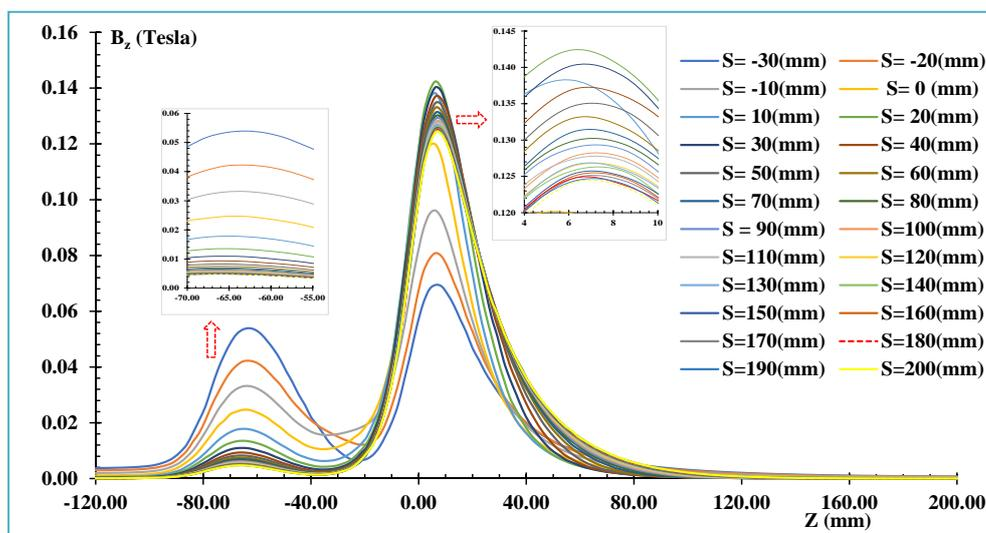
**Fig. 2: Comparison of Axial Magnetic field distribution with iron shroud position with respect to the polepiece**
