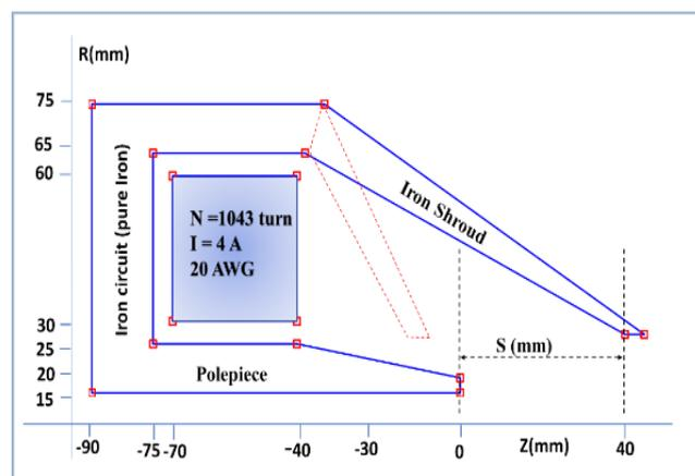
**Fig. 1: The design of snorkel lens with its geometrical parameters**
