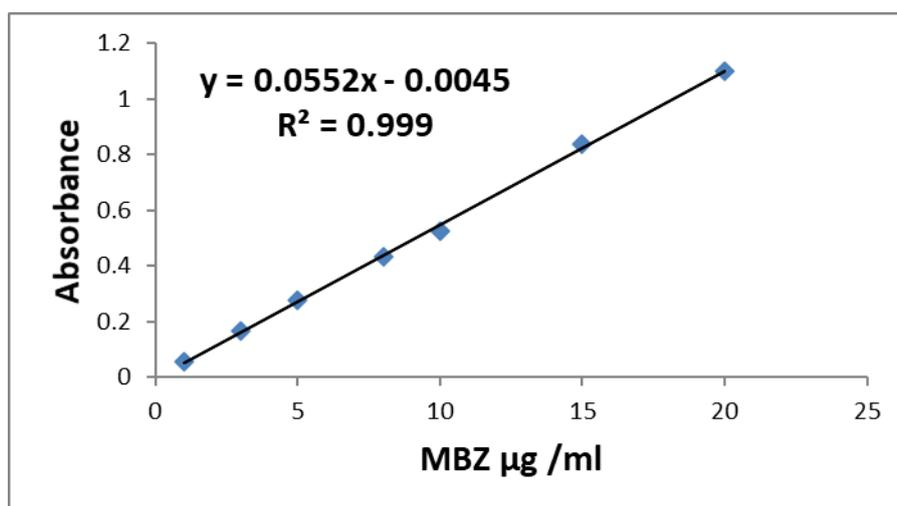
**Fig. 2: Calibration curve of MBZ proceed according to suggested method**
