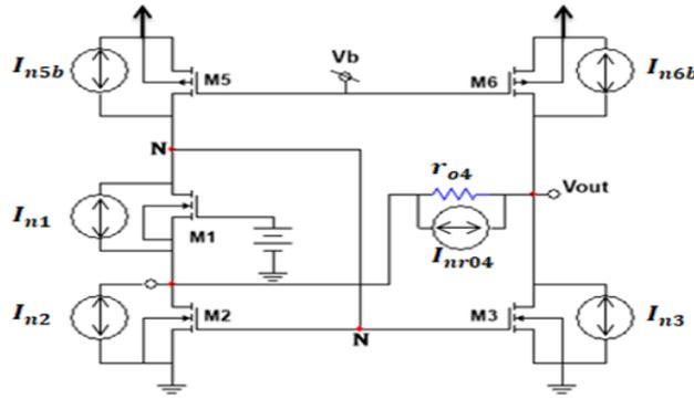
**Fig. 11: Noise sources within the proposed transimpedance amplifier**
