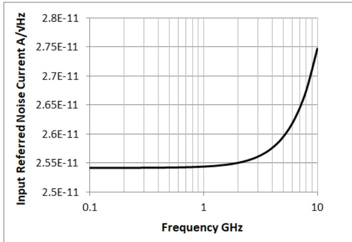
**Fig. 13: Simulated input-referred noise of proposed TIA**
