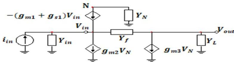
**Fig. 4: Small-signal circuit of the transimpedance amplifier**
