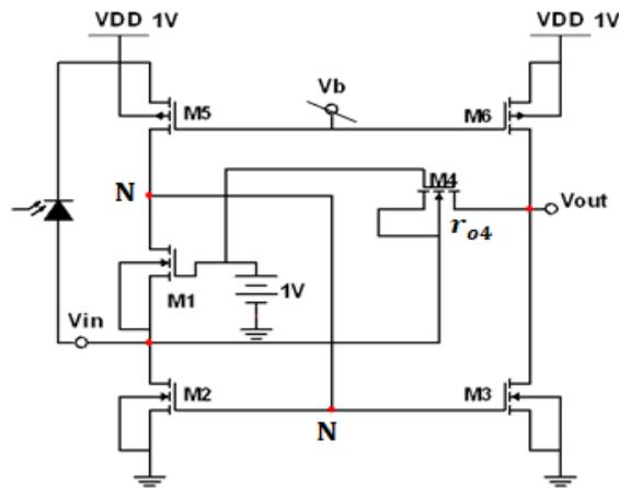
**Fig. 3: Proposed low-voltage optical preamplifier**
