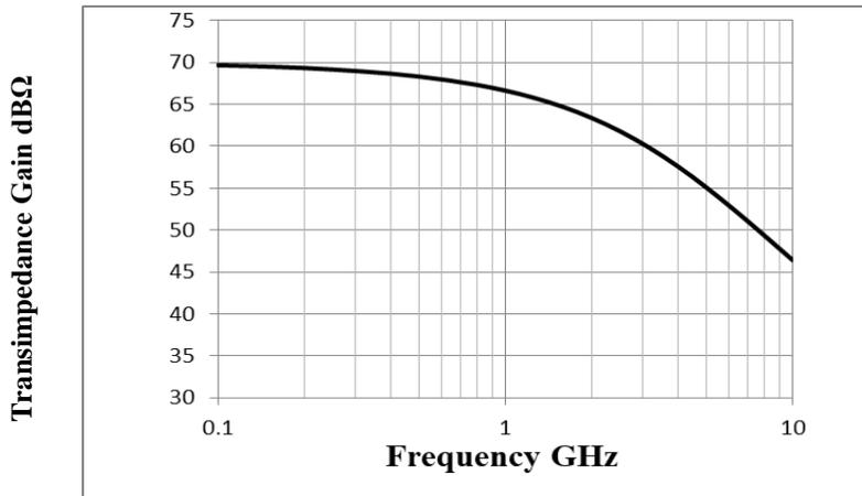
**Fig. 10: Transimpedance gain of the proposed TIA**
