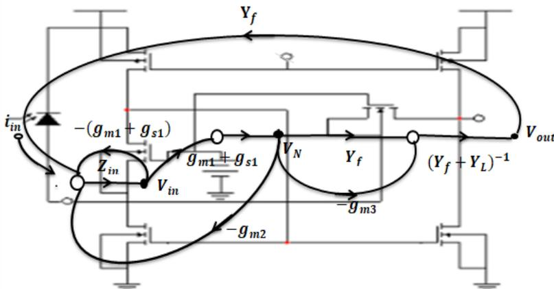
**Fig. 5: Simplified SFG for the signal path**
