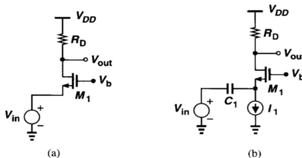
**Fig. 2:(a) (CG)with direct coupling at input.(b) (CG)stage with capacitive coupling at input**
