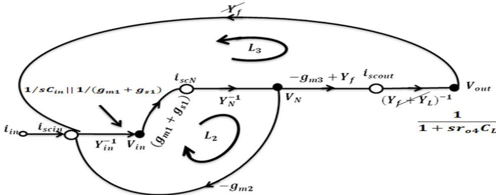
**Fig. 7: Simplified SFG for the signal path**
