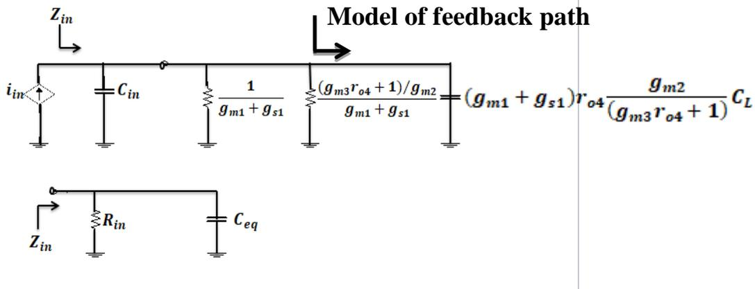
**Fig. 9: Input impedance representation of the proposed TIA.**
